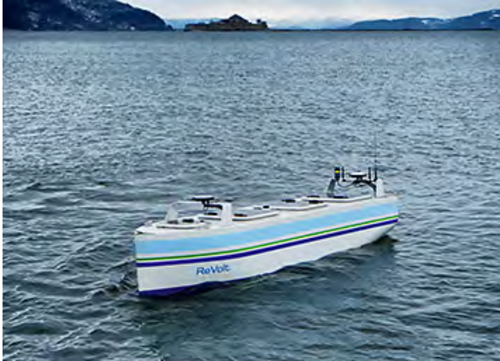
Figure 5. Working scaled model (1:20) of ReVolt concept
